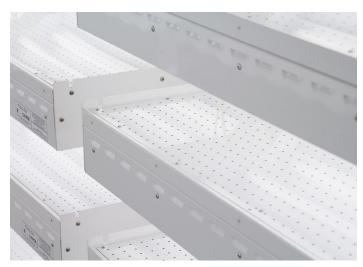
Uniform vertical airflow ensures a precise volume of air is directed upward to avoid condensate buildup on petri dishes.
