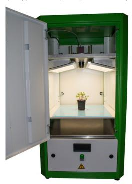
Top-view imaging with incident light from top and/or light box for bottom illumination.
