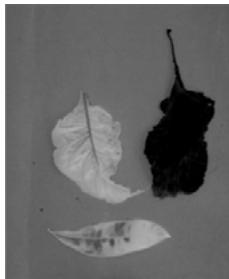
Combining red and infrared image (color-coded visualization of reflectance) to NDVI image (greyscale intensity of NDVI values: light-grey high NDVI, dark-grey low NDVI)
