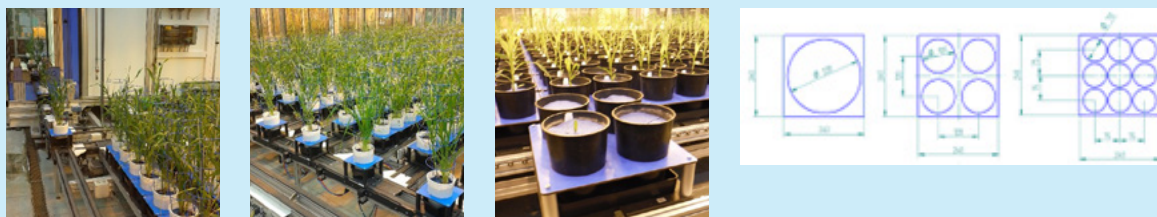
Pots in carriers on conveyor systems with imaging cabinets; carriers can have adaptors for one or more pots.
